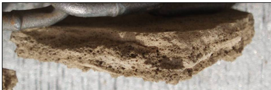
Figure 3. Surface clod from site 148 (a bare patch of soil within a fenced off clay pan). A firmly packed layer of fine sand/silt, approximately 10 mm thick is evident, with an underlying vesicular layer.
